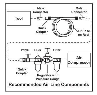
Incorporate a filter, regulator, in-line oiler, shut-off valve, and quick coupler with pressure gauge, and filter for best service, as shown in the diagram above. An in-line shutoff valve is an important safety device to control air flow because it controls air supply in the event of an emergency or even if the air hose is ruptured.
